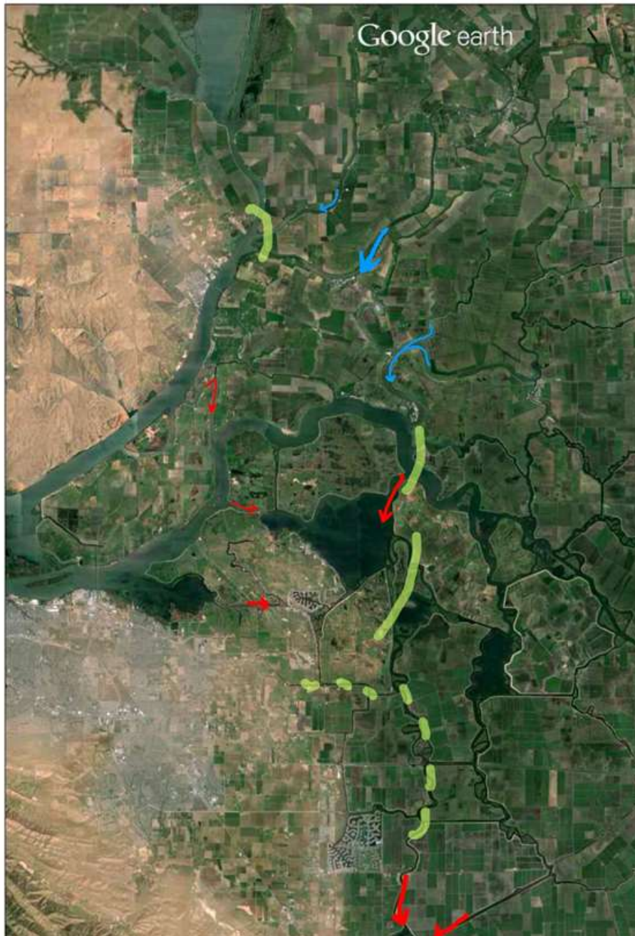
Figure 20. Location of LSZ in summer 2014. The upper boundary of the LSZ is depicted by green boundaries on the lower Sacramento and San Joaquin rivers and Central Delta on Old River. South Delta export water is drawn from the LSZ from areas characterized by net negative flow (red arrows). Export water is replaced by incoming warm, fresh, low turbidity water from the Sacramento River (blue arrows).
